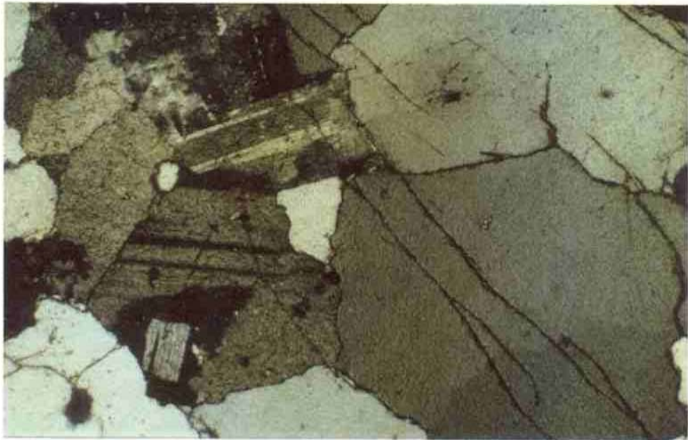
Figure 13. Typical thin slide micrograph of concrete core No4 showing no evidence of AAR.
