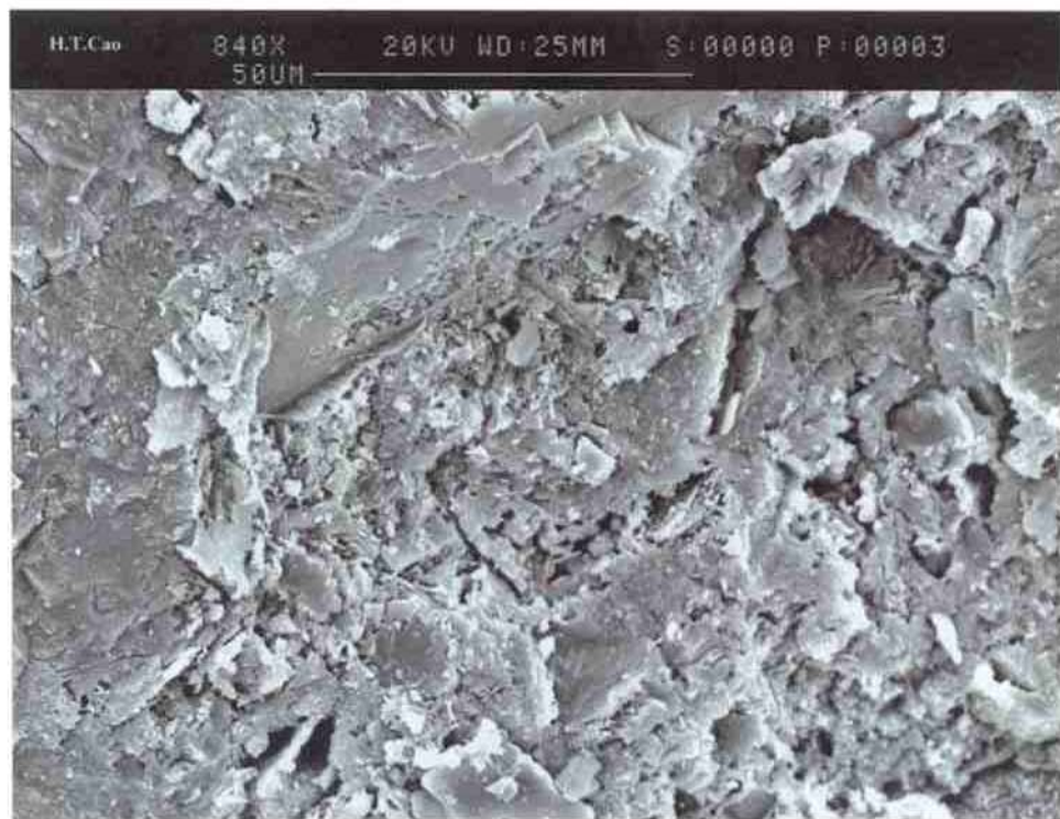
Figure 8. Amorphous “glassy looking” very low calcium – silicate compound (product of Radcon Formula #7) found in the first few mm from treated surface
