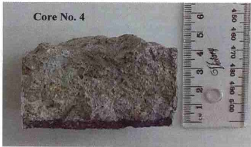
Figure 4. Water penetration after 24 hours in Core No. 4
