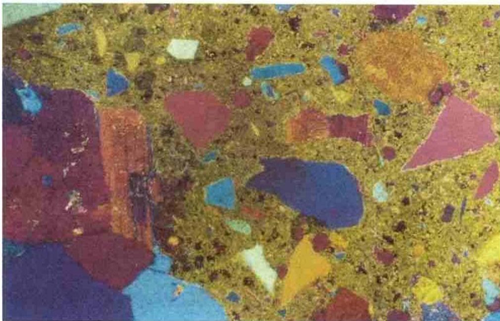
Figure 14. Some thin slide micrograph of concrete core treated with Radcon Formula #7
