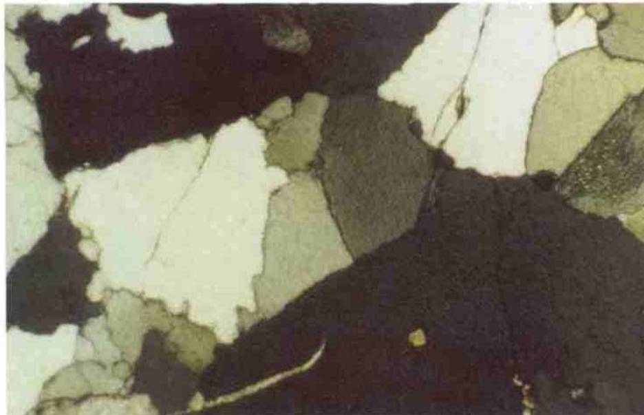
Figure 12. Typical thin slide micrograph of concrete core No3 showing no evidence of AAR.
