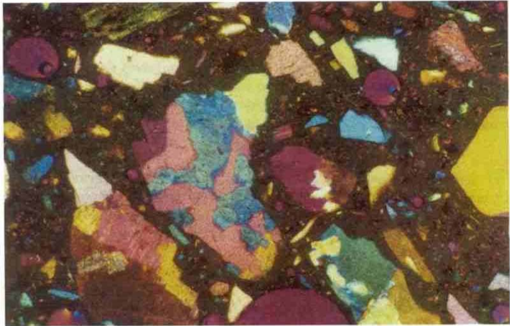
Figure 15. Some thin slide micrograph of concrete core treated with Radcon Formula #7
